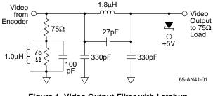
Figure 1. Video Output Filter with Latchup Protection Diode
